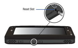
Firmly insert the soft plastic tip of the included Stylus into this slot or until the device exits the current screen and cycles power to the device (turns off then back on) (page 4).
